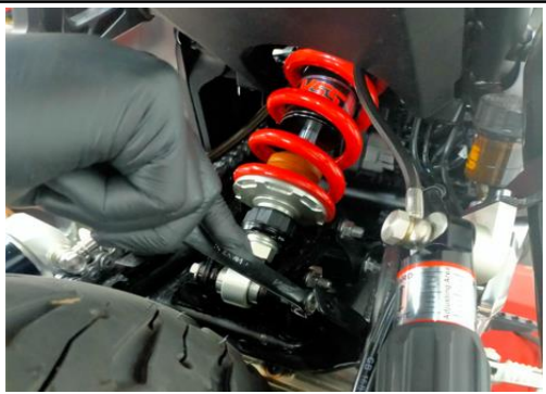
1. INSTALL THE YSS SHOCK ABSORBER AND MOUNT THE TOP AND BOTTOM BOLTS WITH TOOL 14 MM
