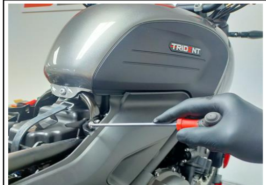
6. ASSEMBLE THE BOTH SIDE OF PANELS WITH HEXAGON TOOL 5 MM
