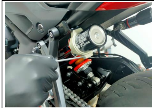
2.. ASSEMBLE THE RESERVOIR WITH THE BRACKET ON THE LEFT SIDE OF BIKE
