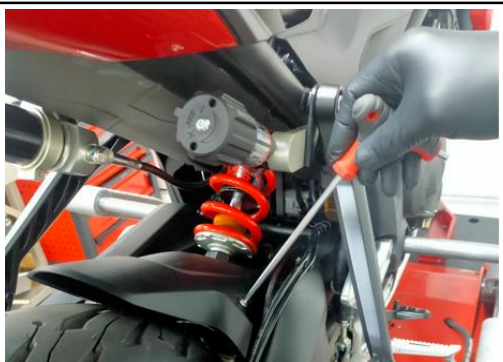
3. ASSEMBLE THE HPA KNOB WITH BRACKET ON THE RIGHT OF THE BIKE
