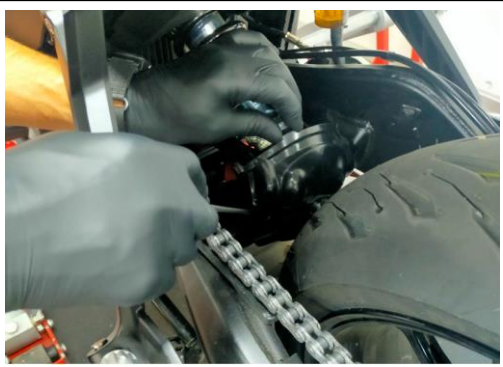
5. REMOVE THE PLASTIC COVER WITH SCREWDRIVER
