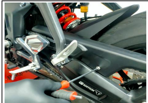
4. ASSEMBLE THE CHAINPROTECTOR AND MUDGARD WITH HEXAGON TOOL 5 MM
