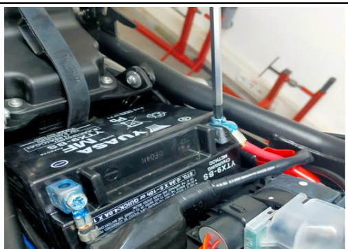
3. DISASSEMBLE THE BOLT FROM BATTERY WITH SCREWDRIVER AND REMOVE THE BATTERY
