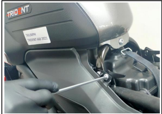
2. TAKE THE BOTH SIDE OF FRAME OFF WITH HEXAGON TOOL 5 MM
