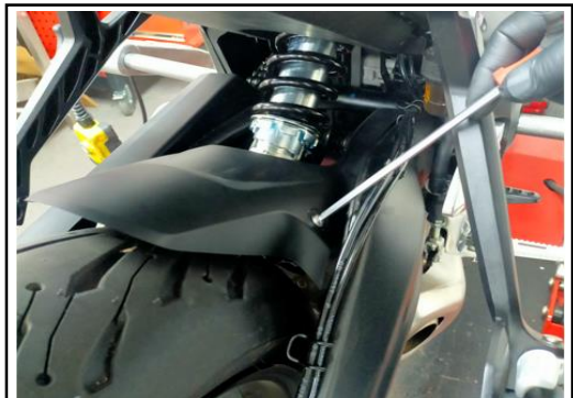
4. REMOVE THE CHAINPROTECTOR AND MUDGARD WITH HEXAGON TOOL 5 MM
