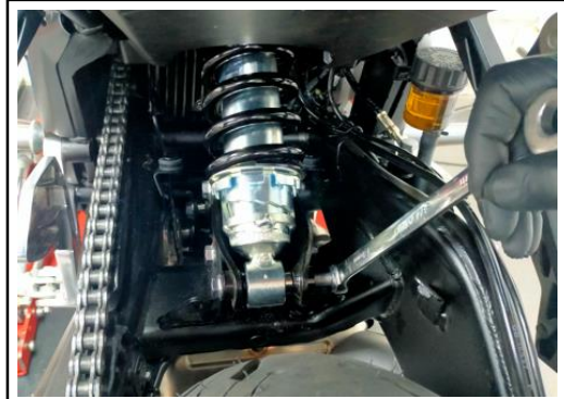
6. DISASSEMBLE THE TOP AND BOTTOM BOLTS FROM THE SHOCK WITH TOOL 14 MM AND REMOVE THE ORIGINAL SHOCK
