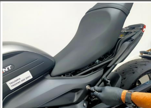
7. ASSEMBLE THE SEAT WITH THE KEY
