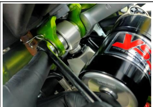
3. ASSEMBLE THE NUT WITH TOOL 17MM AND 19MM
