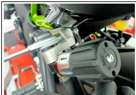
5. ASSEMBLE THE HPA RESERVOIR WITH DELIVERED BOLTS M8
