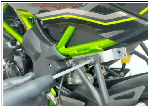
4. TAKE THE HPA BRACKET PLATE, AND ASSEMBLE THIS BETWEEN THE FEETREST AND THE FRAME WITH HEXACON TOOL 6MM.
